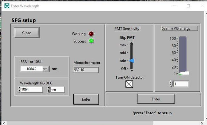
Sfg setup panel- for selecting VIS (SFG)/ 1064 (SHG) , PMT sensitivity, and wavelength (532 (SFG) or 1064 (SHG))
