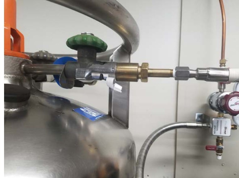
Close green valve and remove gas line, remember lefty loosey righty tighty
