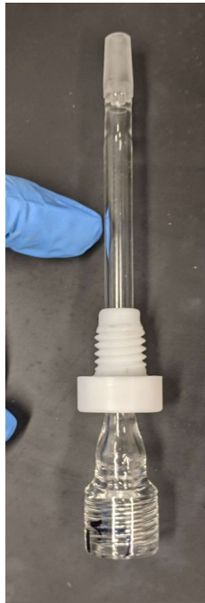
2. Attach threaded Kel-F vacuum adapter to the plunger
