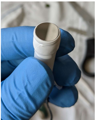
1. Wrap the W.E. to Kel-F bottom piece with Teflon tape
