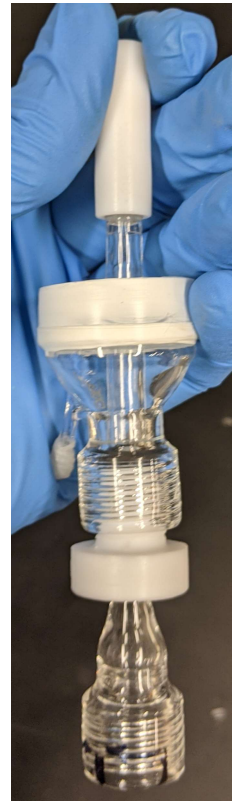
5. Attach the Kel-F piece to the end of the plunger
