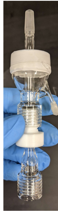
4. Attach the glass cell & tighten it to the threaded Kel-F vacuum adapter with the rubber piece in between to seal it
