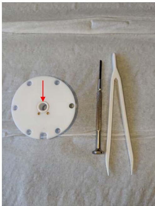
Install Teflon gasket in bottom of Teflon cell base
