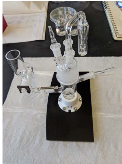
Leak test before installing on VeeMax
