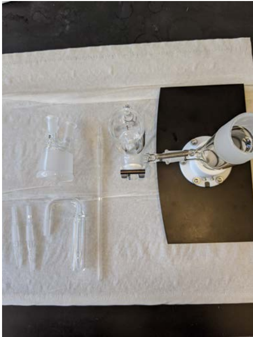
Install cap, bubbler wand, purge inlet, counter electrode holder, and exhaust bubbler
