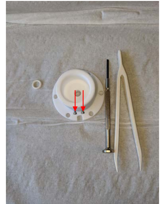
Depress pogo pin and tighten screw to keep flush with cell bottom
