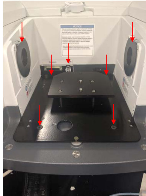
Install ATR bracket in sample chamber • Attach accessory connector to back of bracket • 7/64 th " hex screw
