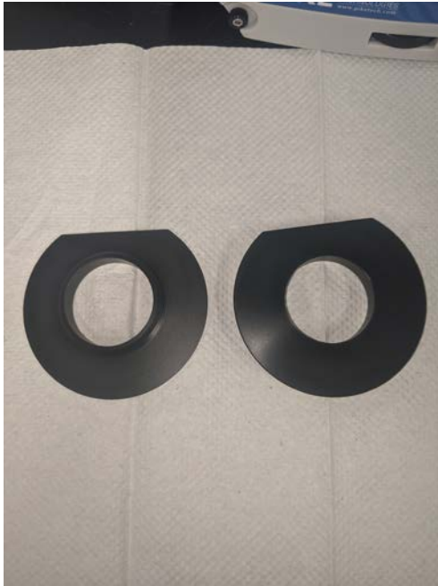
Install gaskets on sides of sample chamber
